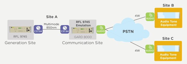
Figure 2: Updated system with fiber optic digital teleprotection
